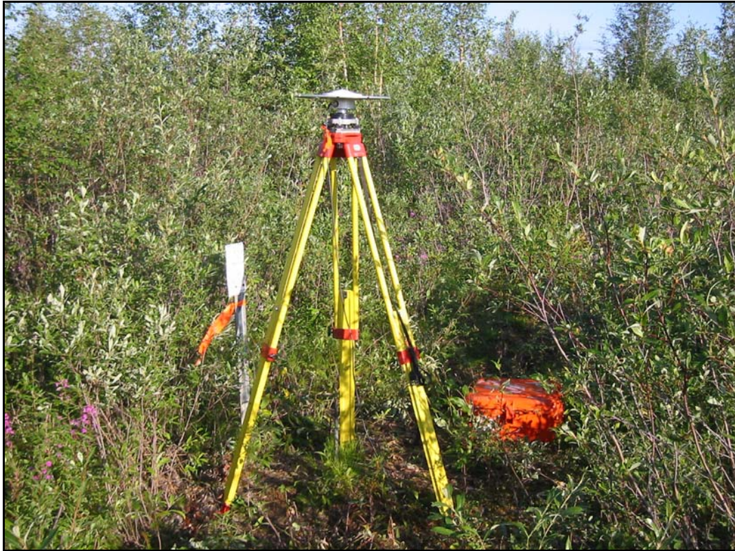
Figure 5.2 Test-bed with a geodetic GPS receiver set over benchmark 623 (2004 campaign). Vegetation in the area was moderately-dense small trees and bushes, with moss below.
